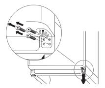
Remove the door fitting from the door bearing (1, 2). Move the bearing pivot from the right to the left hand hole (3). Place the door fitting supplied on the bearing pivot (4, 5).
